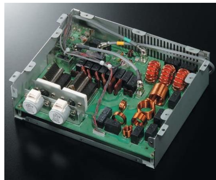
●Automatic, High-Speed 500-Watt-Capable Antenna Tuner
