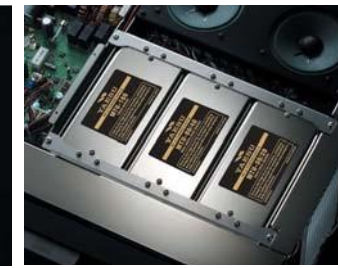
● Three \mu -Tune Modules Installed in FT DX 9000 Mainframe
