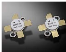
●200-Watt Version Utilizes Push-Pull SD2931 Devices
