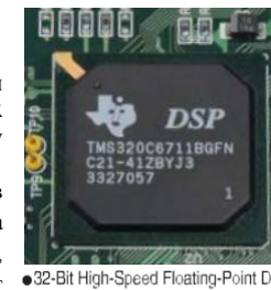
● 32-Bit High-Speed Floating-Point DSP
