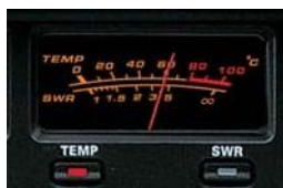
●Final Amplifier Temperature Display (MP/Contest Versions)
