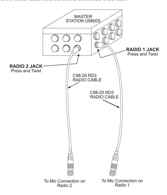
**Note:** Do not connect to the radio's rear panel command mic connectors. On the IC-M602, you must connect to the front mic connector. On the IC-M604, you must connect to either the front mic connector or the rear pig-tail mic connector (preferred).
